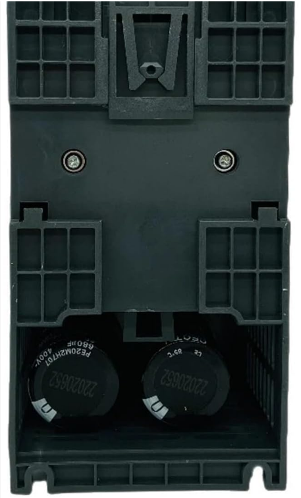
Figure 3: Rear view of the VFD, illustrating the mounting points and internal capacitor components.
