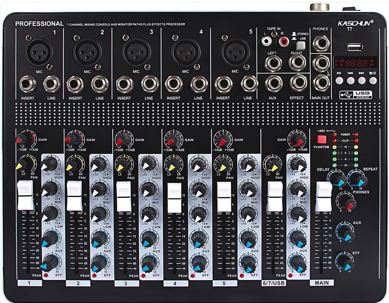
Figure 1.1: Front view of the Kaschun T7 Professional Audio Mixer, showcasing its 7 channels, various inputs, faders, and control knobs.
