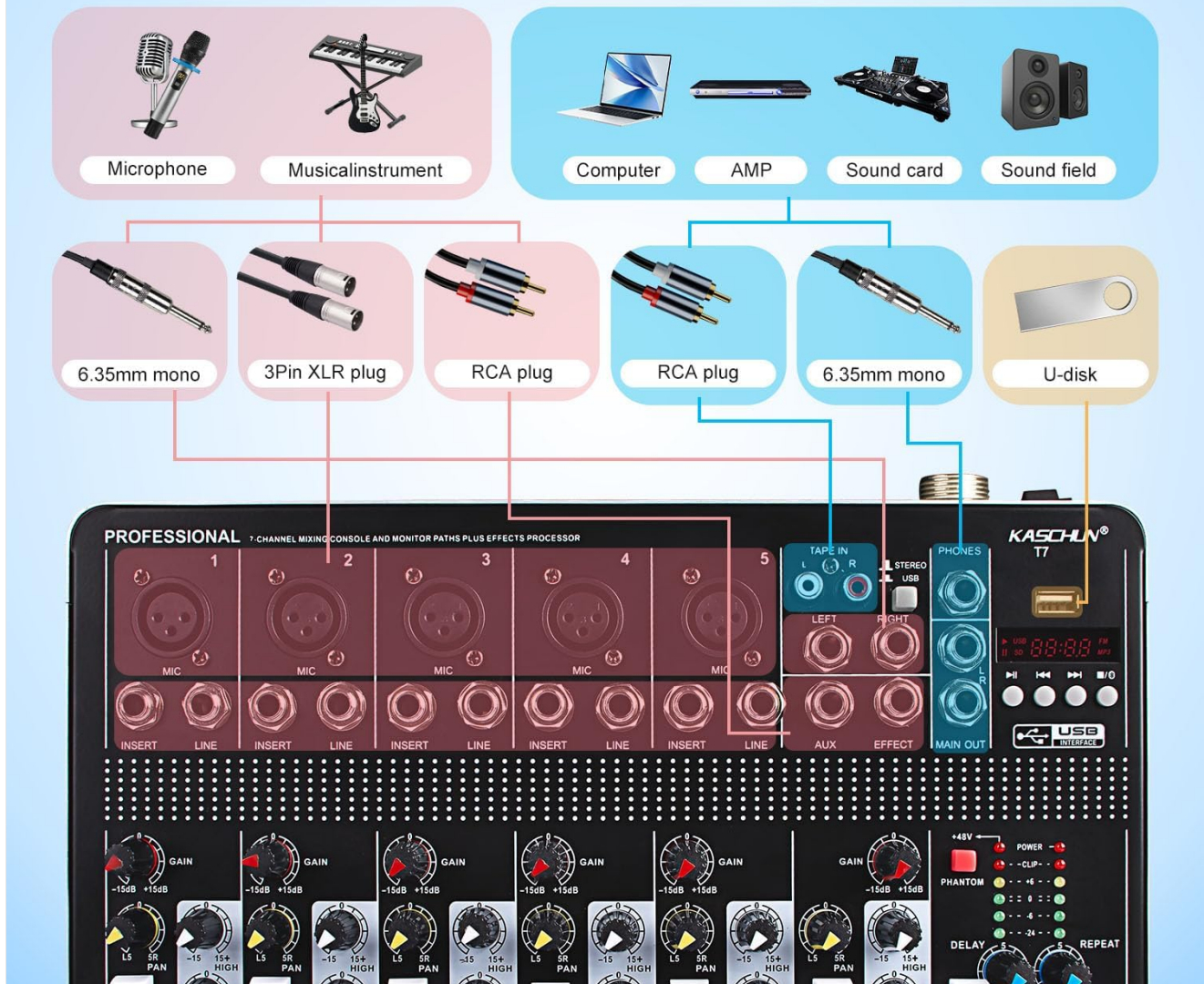
Figure 3.2: The mixer supports multiple device connections, including microphones, musical instruments, computers, and various audio equipment using 6.35mm mono, 3-pin XLR, and RCA plugs.
