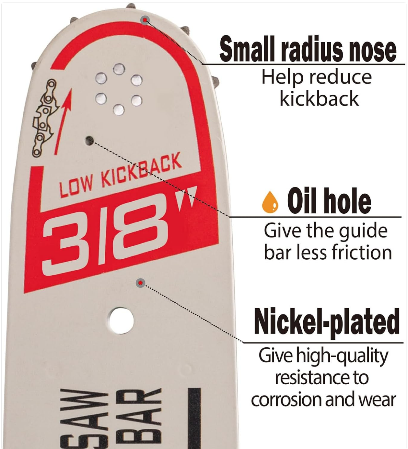
Figure 4: Key features of the guide bar, including the small radius nose for reduced kickback, the oil hole for lubrication, and nickel-plated surface for corrosion resistance.
