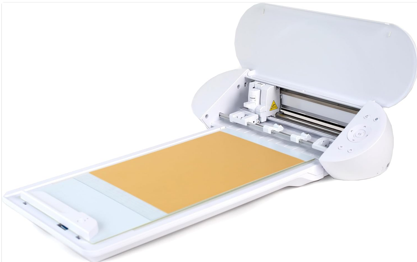
Image 3.1: The Silhouette Electrostatic Mat loaded into a Portrait 4 machine, with a piece of material placed on its surface, ready for cutting.
