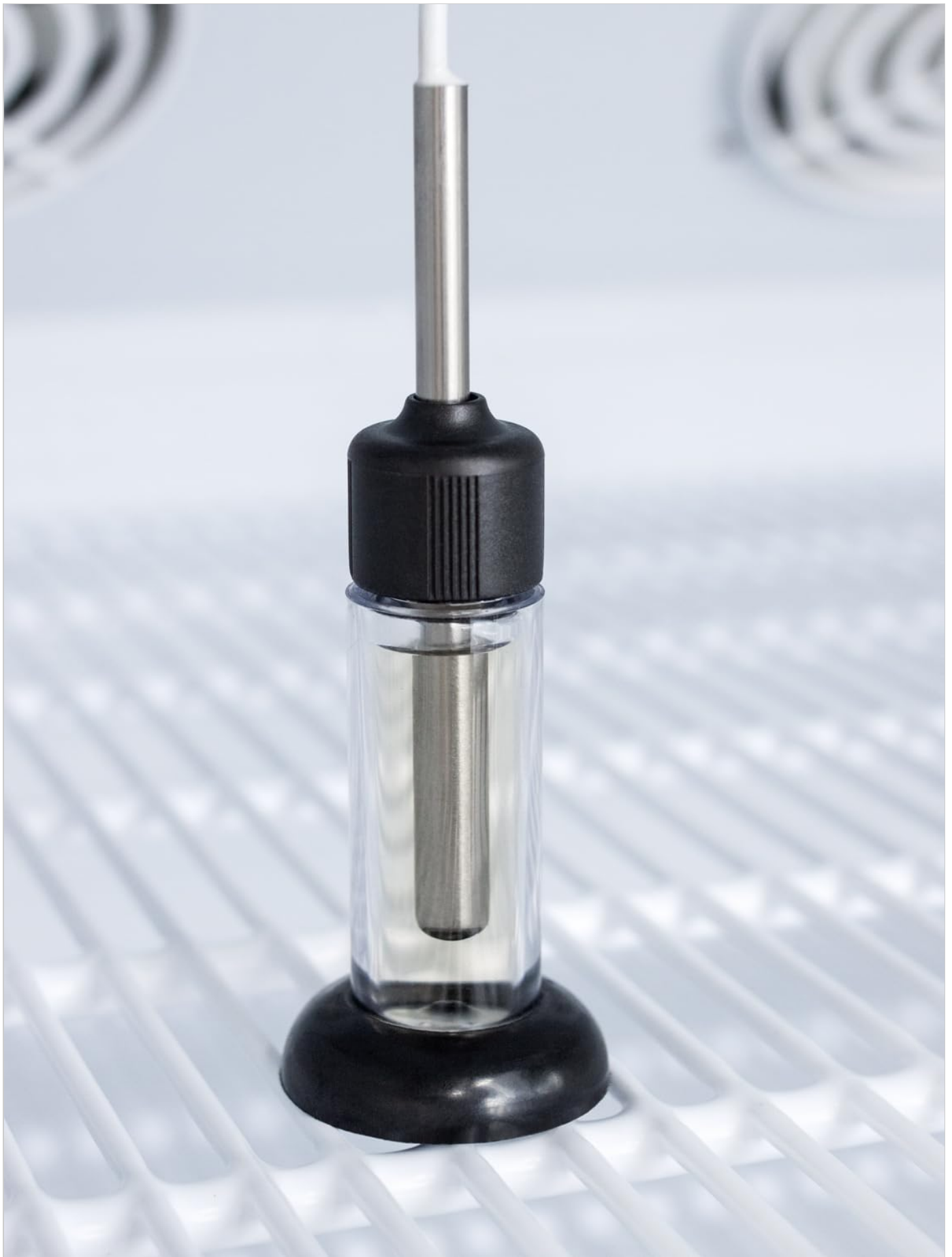
Figure 3: Temperature probe within a glycol-filled vial, used for accurate temperature monitoring inside the unit.
