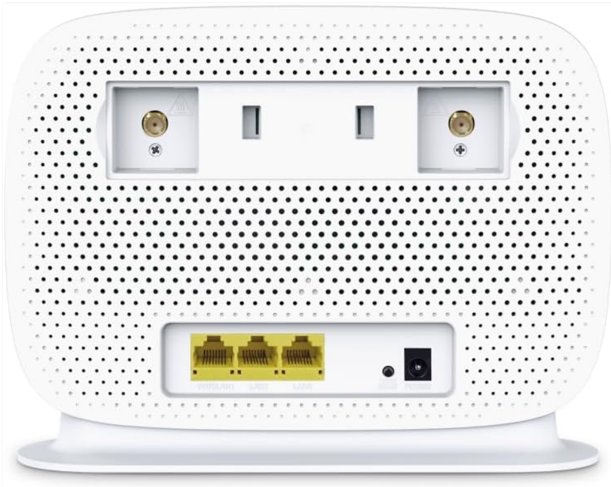
Figure 4: Rear panel of the Archer MR505 with ports and SIM slot.
