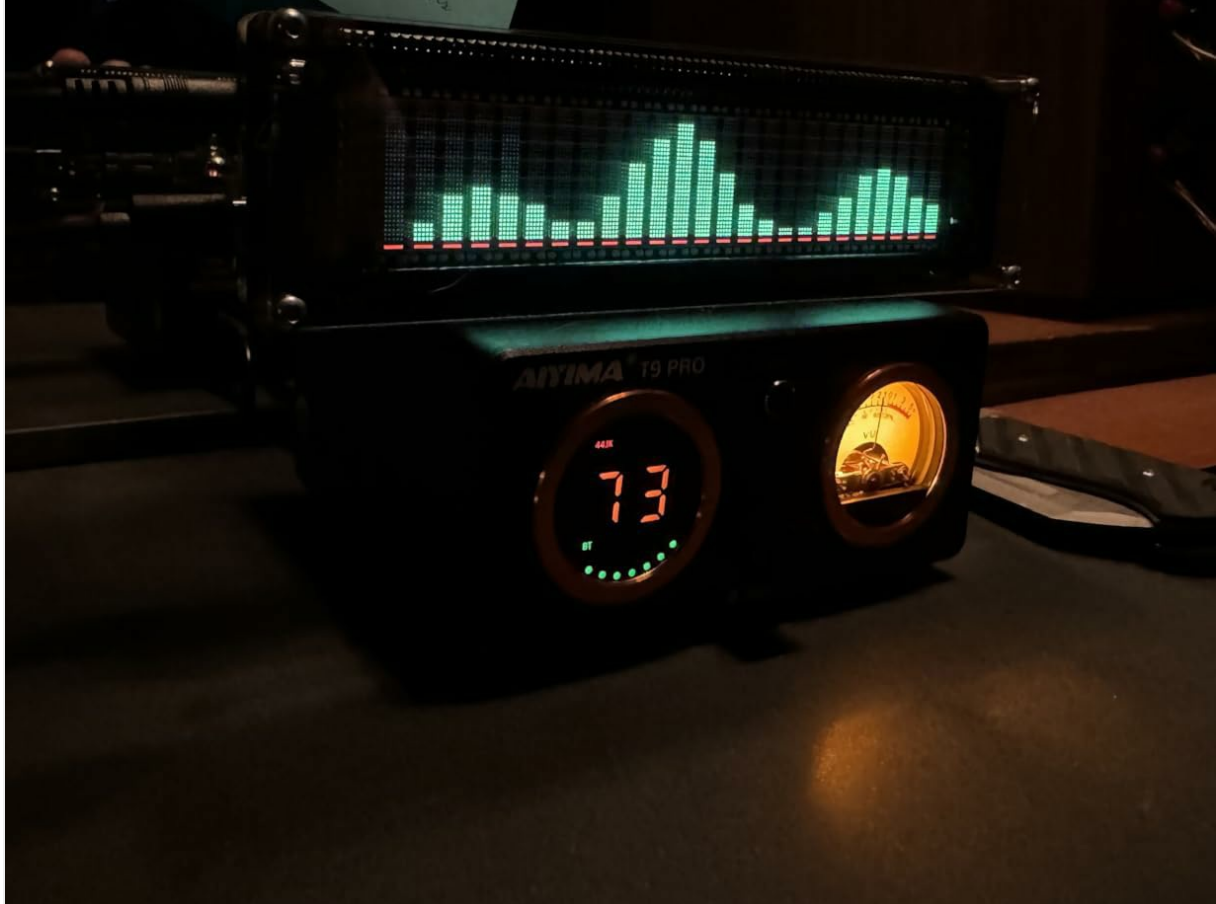
Image: The AK2515 displaying a wide frequency sweep, demonstrating its audio analysis capabilities.
