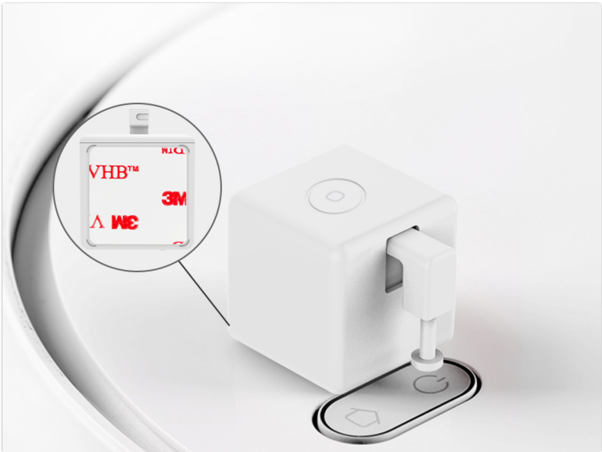
Image: The underside of the Fingerbot showing the 3M VHB adhesive tape for secure mounting.
