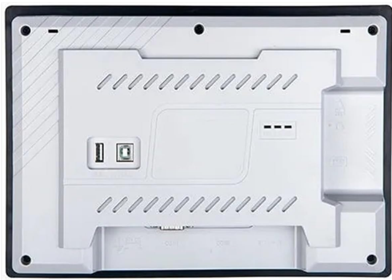
Figure 2.3.1: Rear view of the LVSEDTAL PI3102IG-C(AG) HMI, illustrating the location of USB ports (Type A and Type B) and serial communication ports.
