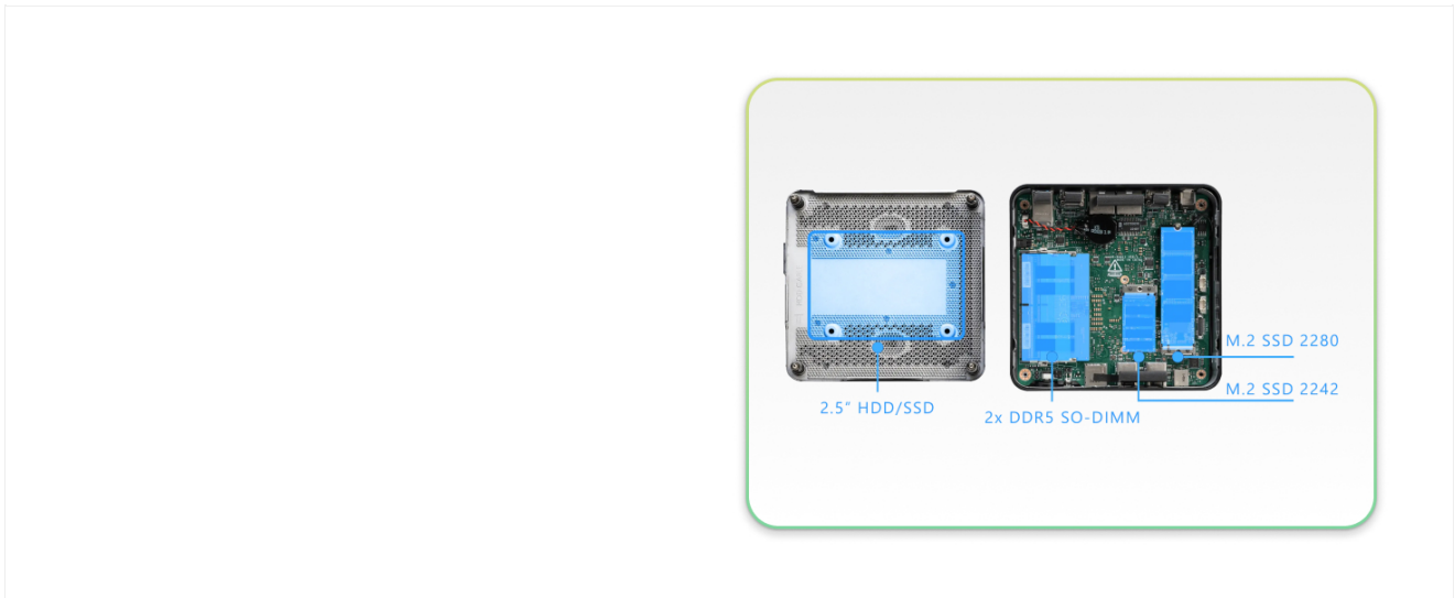
Figure 5: Internal components and upgrade options.
