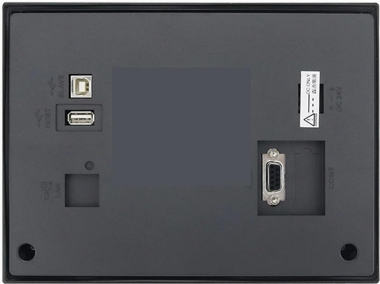
Figure 2.2: Rear view of the HMI, illustrating the DC 24V power input, COM2 port, USB Host, USB Slave, and LAN port.
