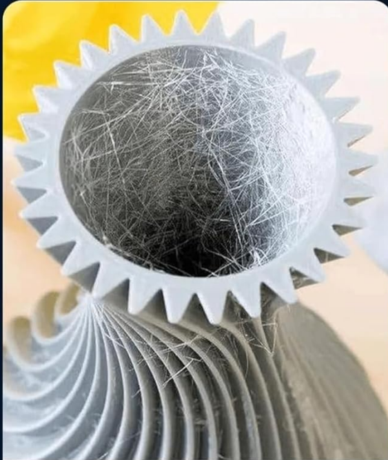
Before (Undried Filament)Stringing/ clogging /poor adhesion/layer shifting
