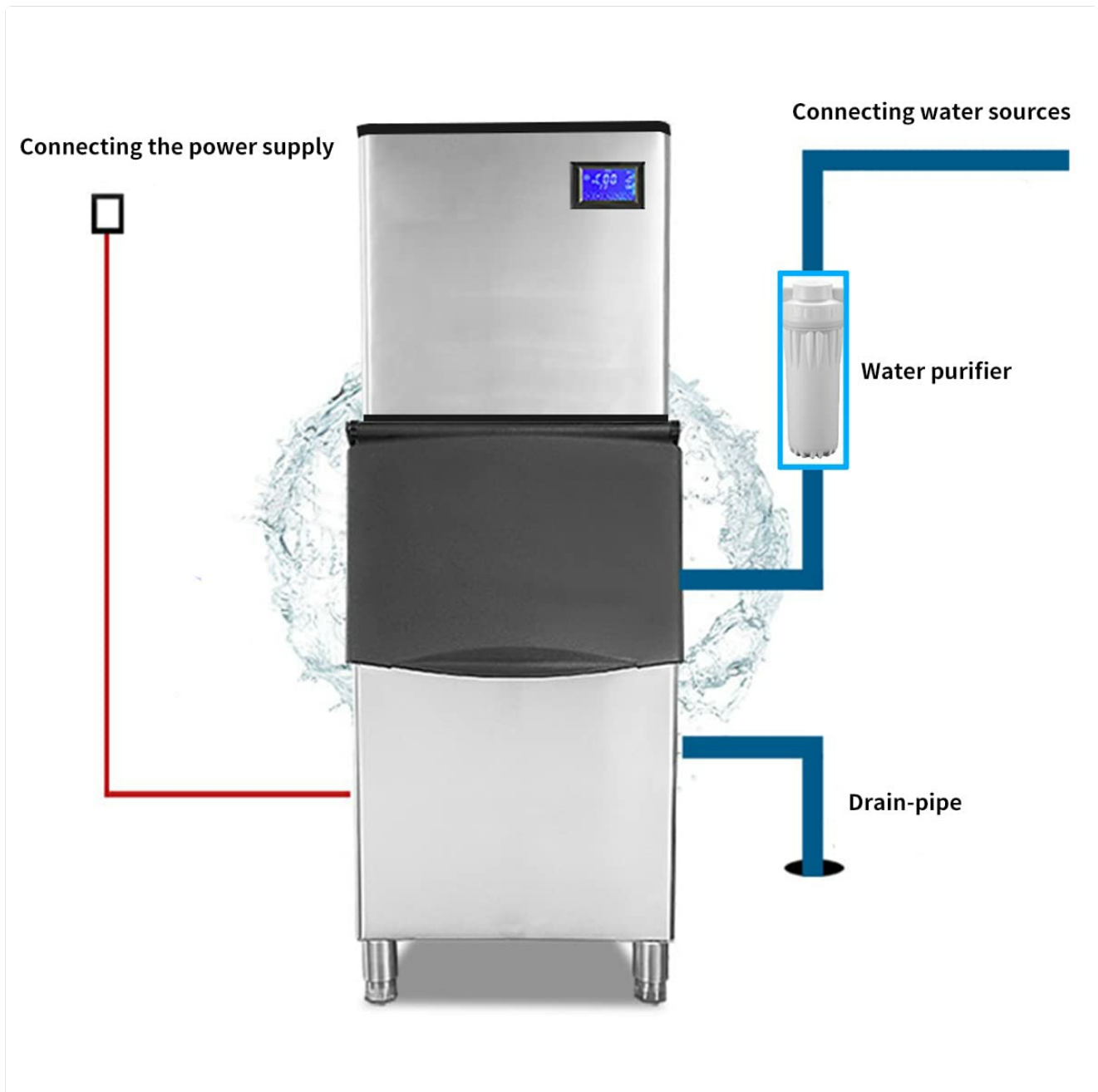
Figure 4.2: Detailed connection points for power supply, water source with purifier, and drain pipe.
