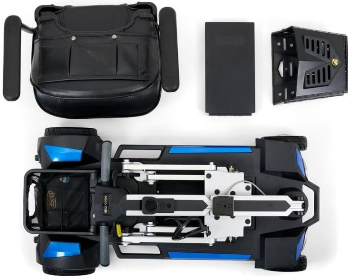
View of the scooter disassembled into its main components: seat, battery, basket, and main frame, for easy transport.
