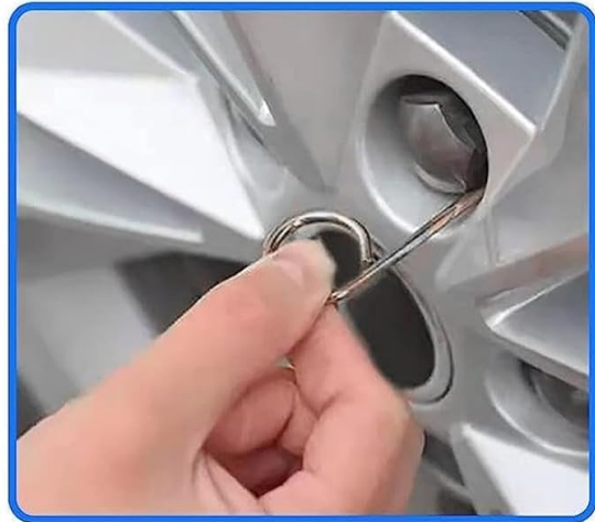
Image: Examples of the black plastic tool and the silver ring tool being used to remove different types of wheel caps.
