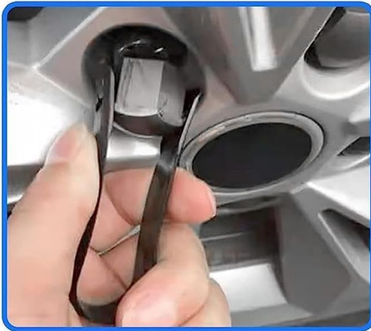
Image: Examples of the black plastic tool and the silver ring tool being used to remove different types of wheel caps.
