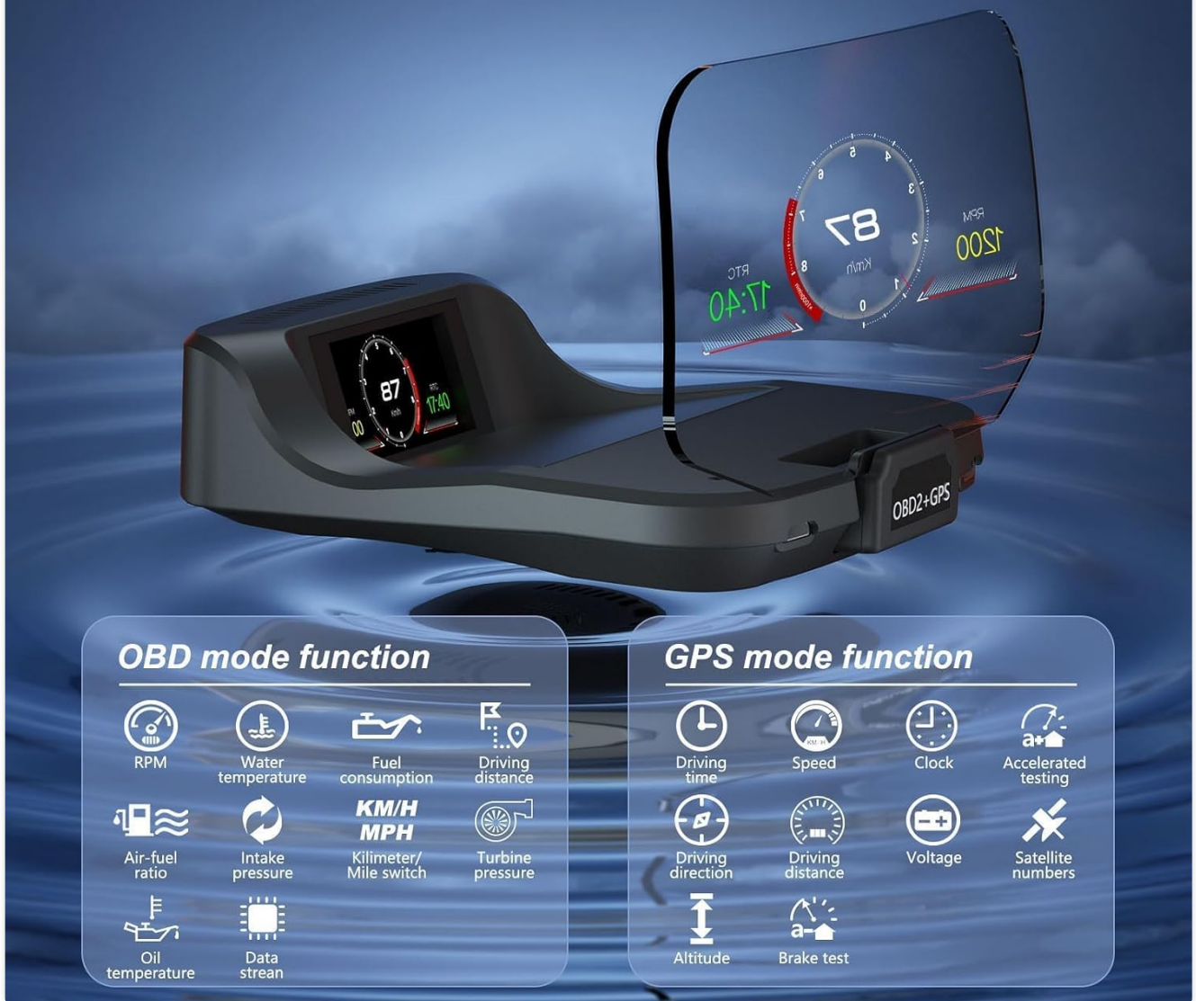
Image 6: A detailed view of the HUD's display, illustrating the distinct data sets available in both OBD and GPS operating modes.
