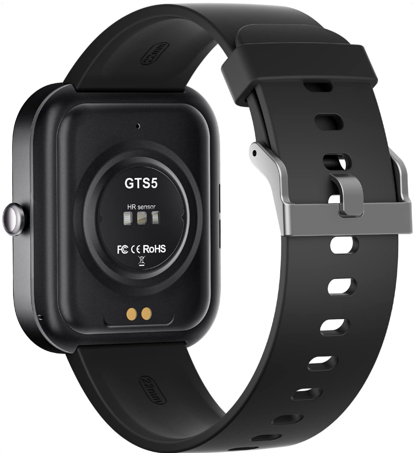
Image 4.3: The rear view of the GTS-5 smartwatch, highlighting the heart rate sensor and charging pins.
