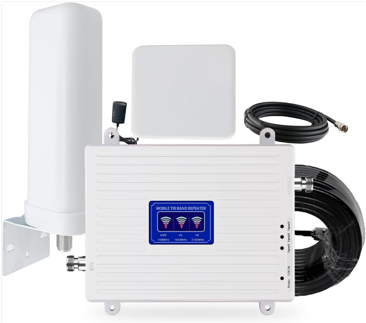
Figure 1: All components included in the Generic Cell Phone Signal Booster kit. This includes the booster unit, outdoor antenna, indoor antenna, coaxial cables, power supply, and mounting hardware.
