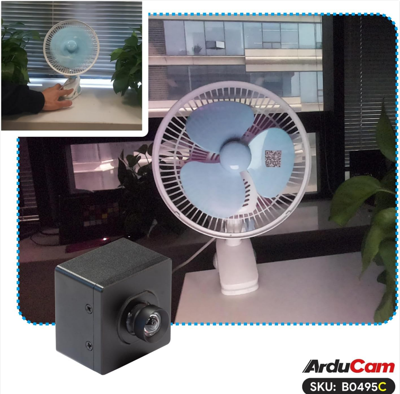
Image 4.1: A spinning fan captured by a global shutter camera, showing no motion distortion on the blades.
