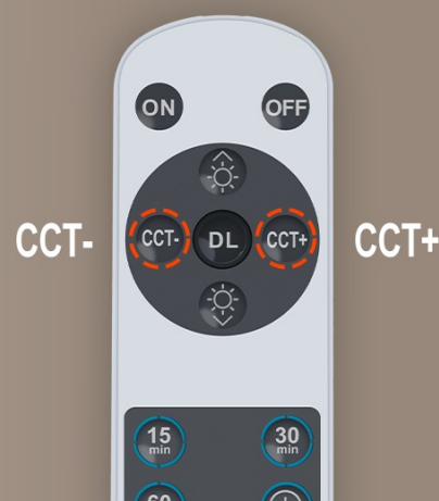
Image: A visual guide showing the range of color temperatures from 2700K to 6000K and how to select them using the CCT- and CCT+ buttons on the remote.
