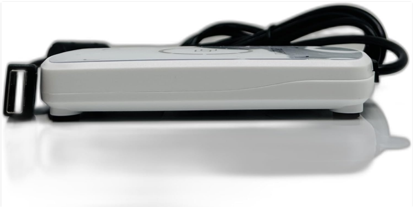
Figure 3: FONGWAH UHF RFID Reader/Writer connected via USB.
