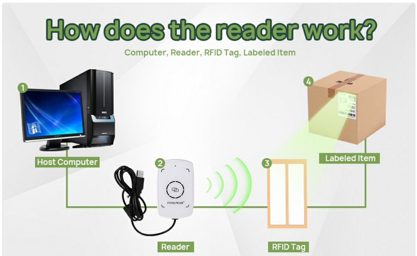
Figure 1: Basic operation diagram of the FONGWAH UHF RFID Reader/Writer.
