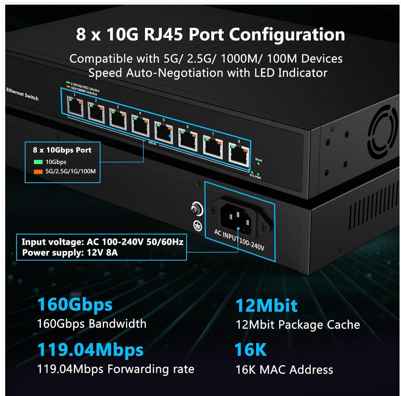
Image 8.1: Key specifications and power input details of the switch.
