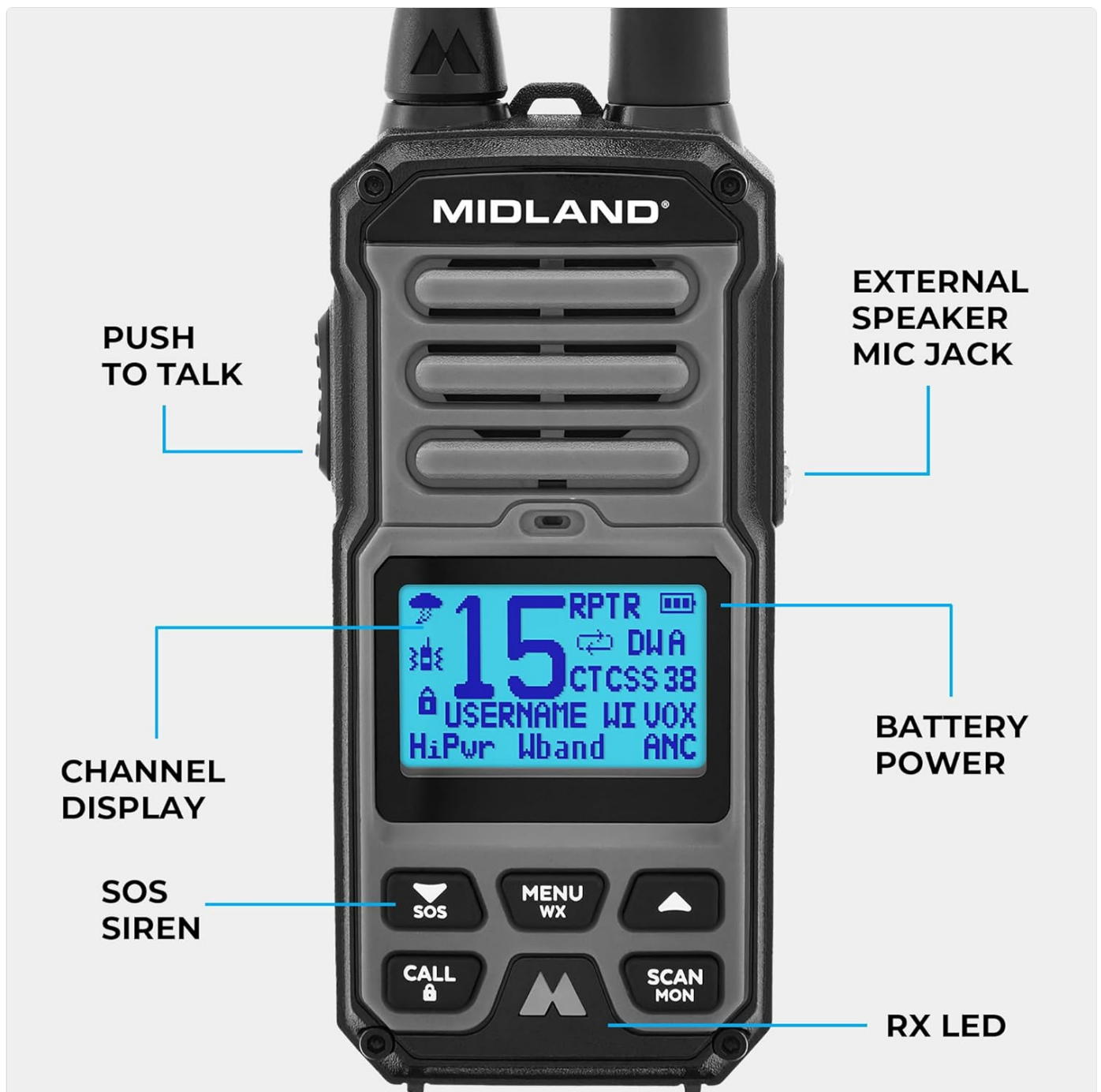
Image: A detailed view of the Midland GXT67 Pro's front panel, highlighting the Push to Talk (PTT) button, Channel Display, SOS Siren, Call button, Menu/WX button, Scan/Mon button, External Speaker/Mic Jack, and Battery Power indicator.
