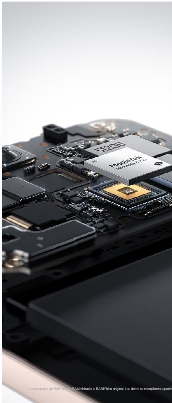
Figure 6: Internal view highlighting the MediaTek Dimensity 6300 processor and memory configuration.
