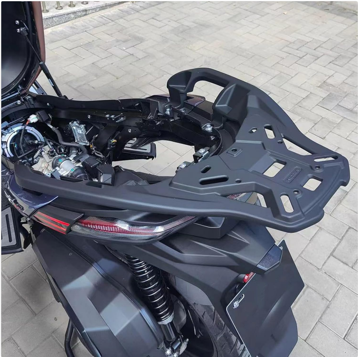
Figure 5.1: Rack positioned on the motorcycle for installation.
