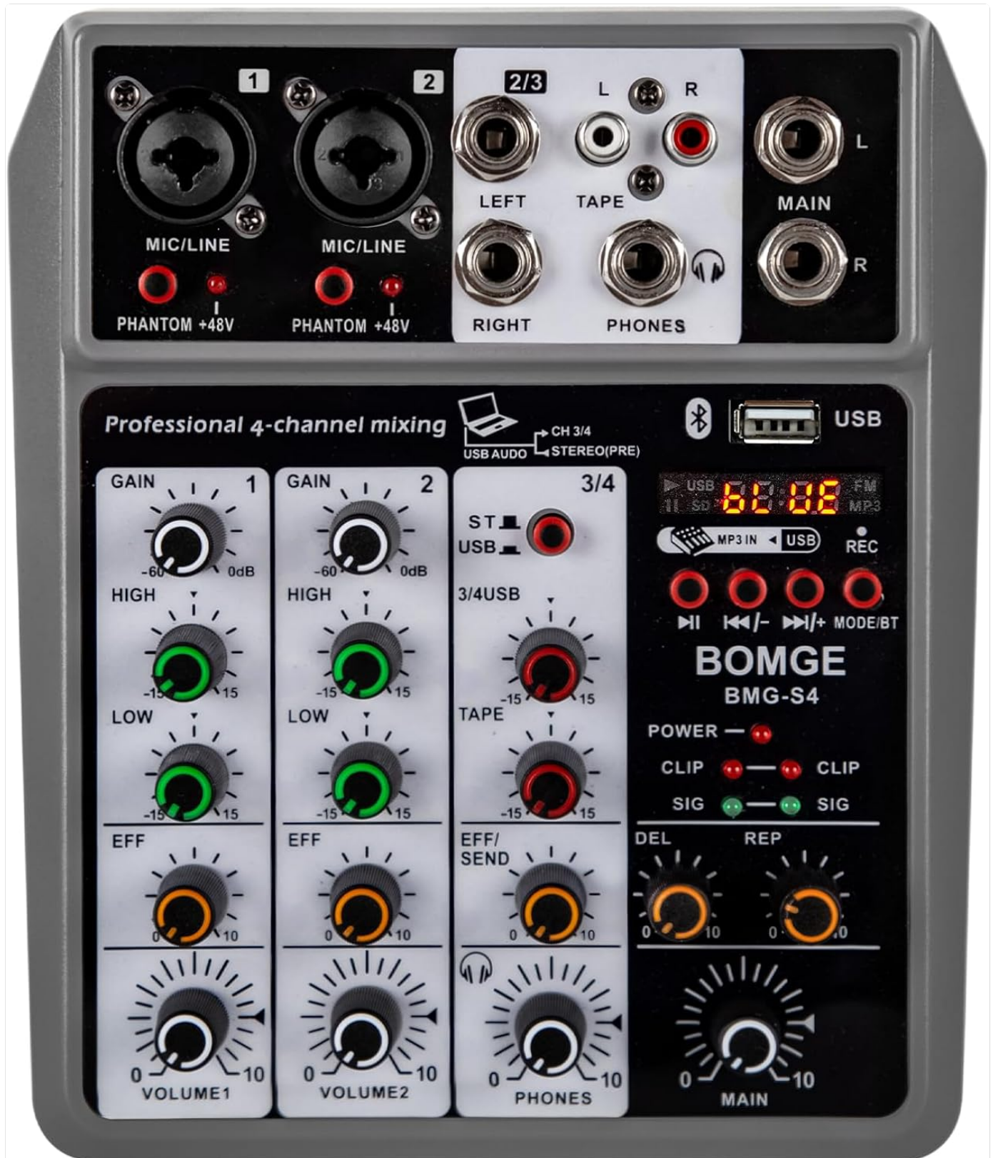
Figure 4.1.1: Front view of the BOMGE audio mixer, showing all knobs, buttons, and indicators.
