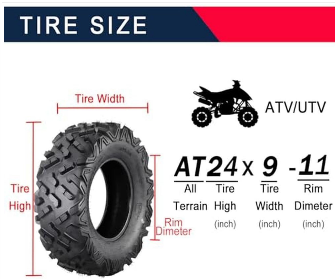
Figure 3.1: Diagram illustrating how to measure tire dimensions, including tire high, tire width, and rim diameter, crucial for proper fitment.
