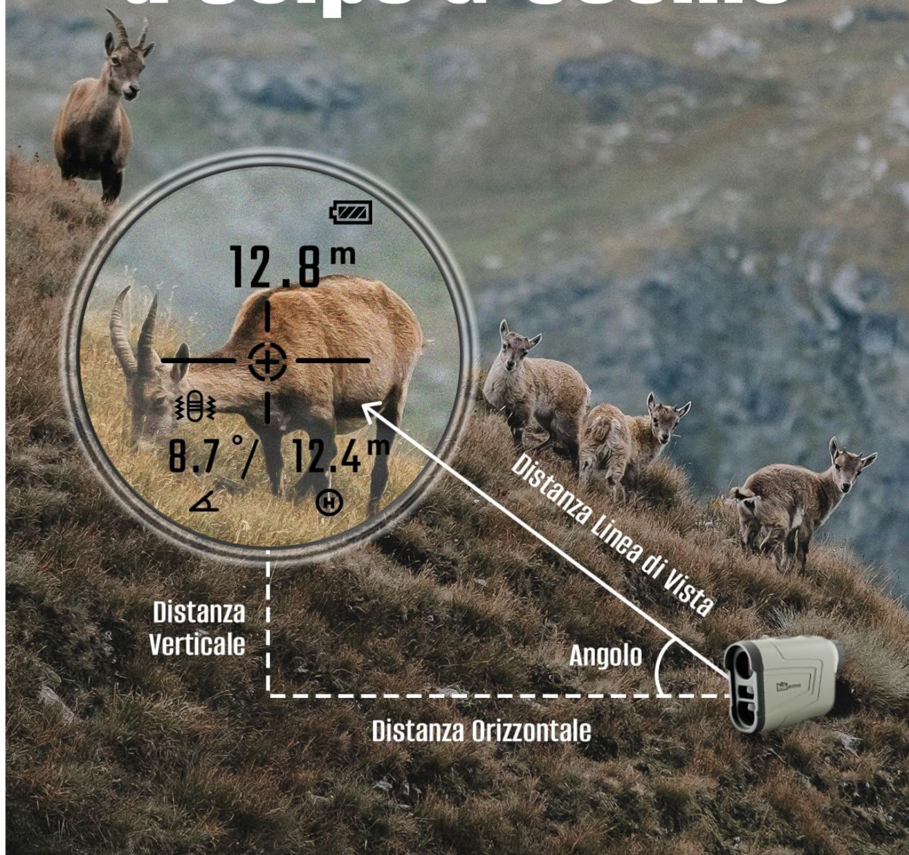
Image: Display showing vertical distance, horizontal distance, and line of sight distance to an ibex on a hillside.
