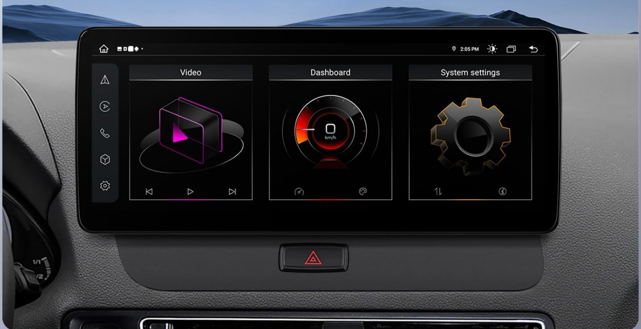
Figure 5: Main Interface. This image shows the main user interface of the XTRONS car stereo, featuring icons for various functions like video playback, dashboard information, and system settings.
