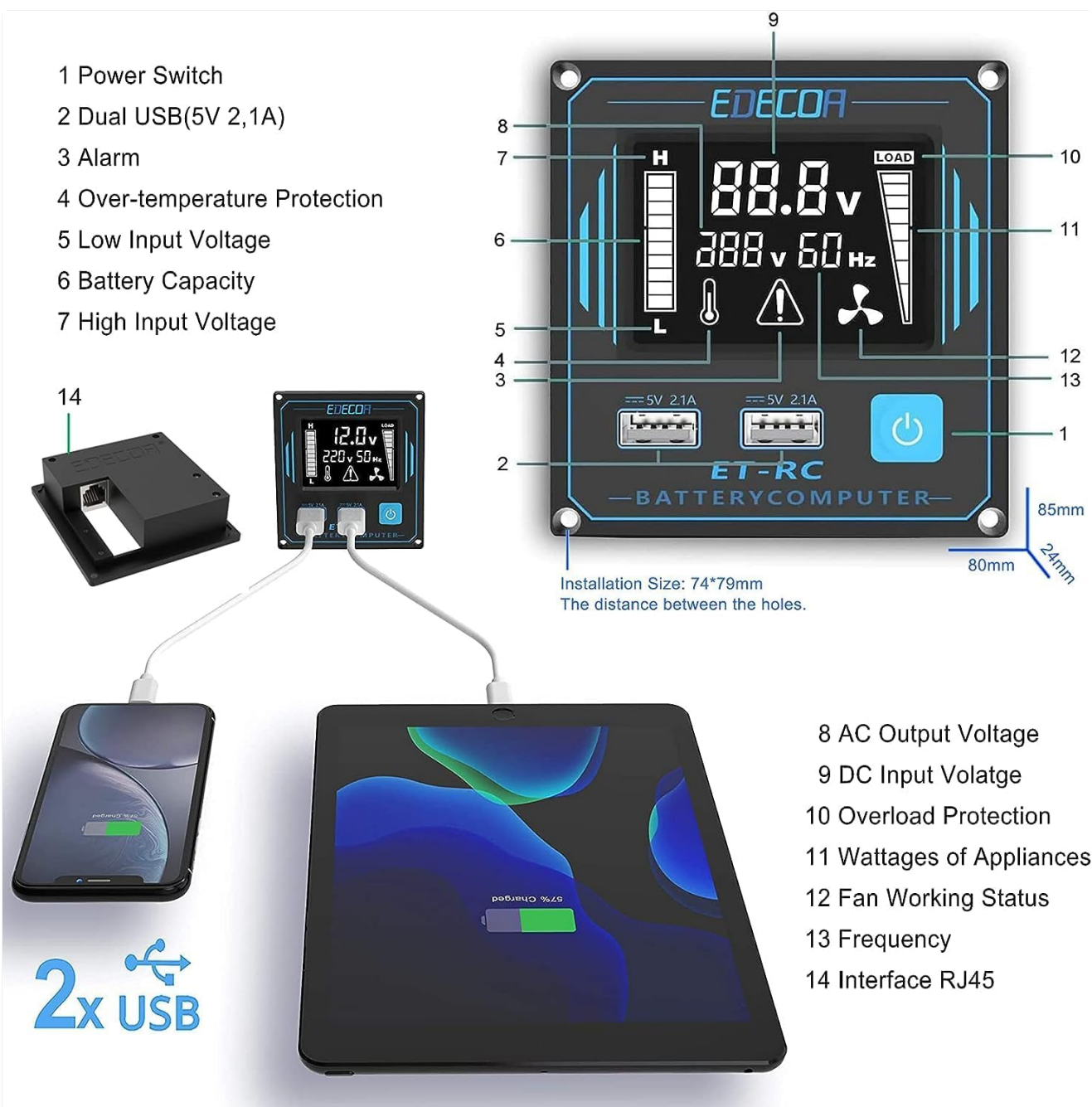
Image 4.2: Detailed view of the ET-RC remote controller display and its various indicators and controls.
