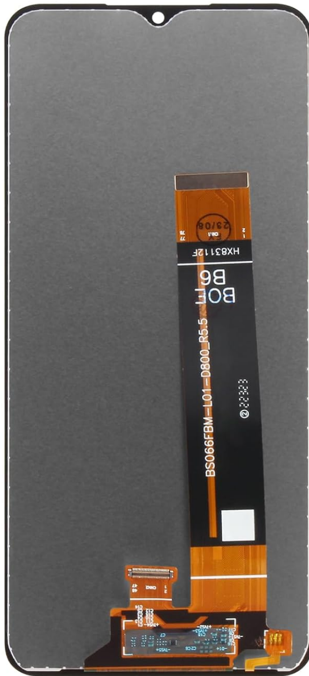
Image: Back view of the LCD screen replacement, highlighting the integrated flex cable and connector for the phone's motherboard.
