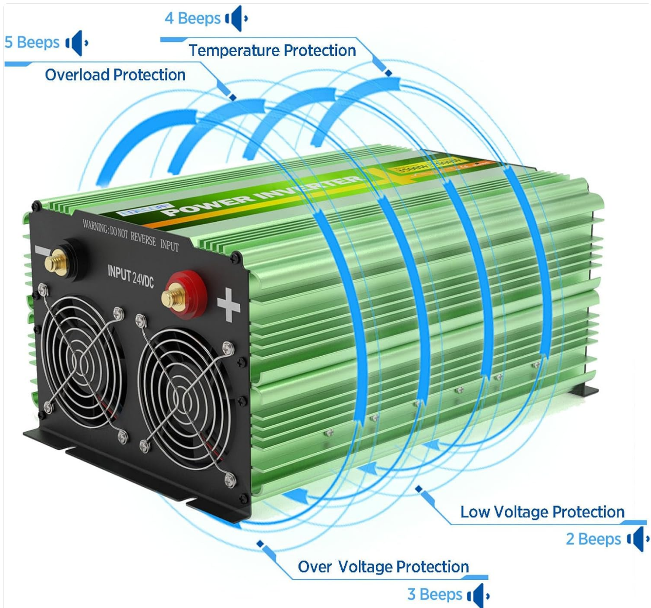
Figure 3.4: Inverter Protection System and Beep Codes.
