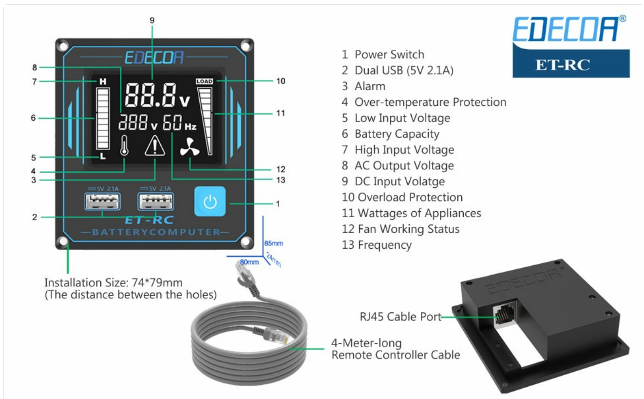
Figure 3.3: ET-RC Remote Controller Display and Functions.
