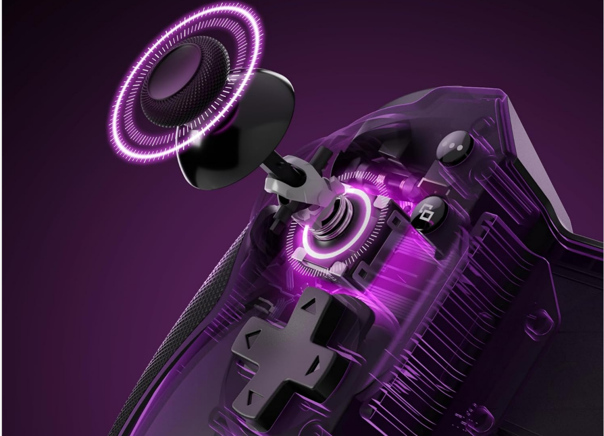
Figure 2.2: Internal view highlighting Hall Effect Joysticks.
