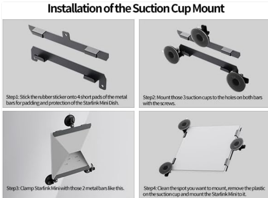
Image: Step-by-step installation guide for the suction cup mount.
