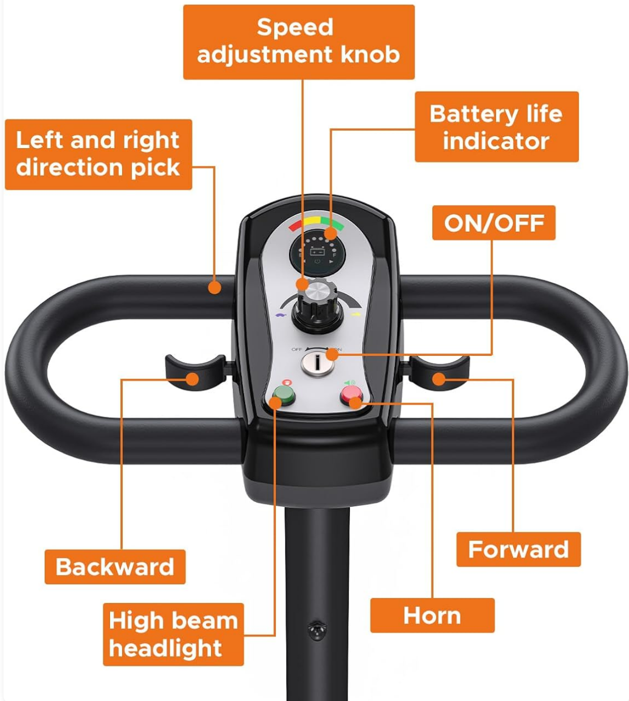
Image 5.1: Diagram of the scooter's control panel, highlighting the speed adjustment knob, battery life indicator, ON/OFF switch, forward/backward controls, high beam headlight button, and horn button.
