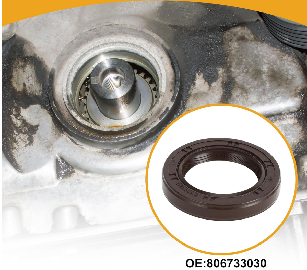
Image 5.1: An example of a crankshaft oil seal in an engine, illustrating its typical installed location near the crankshaft.
