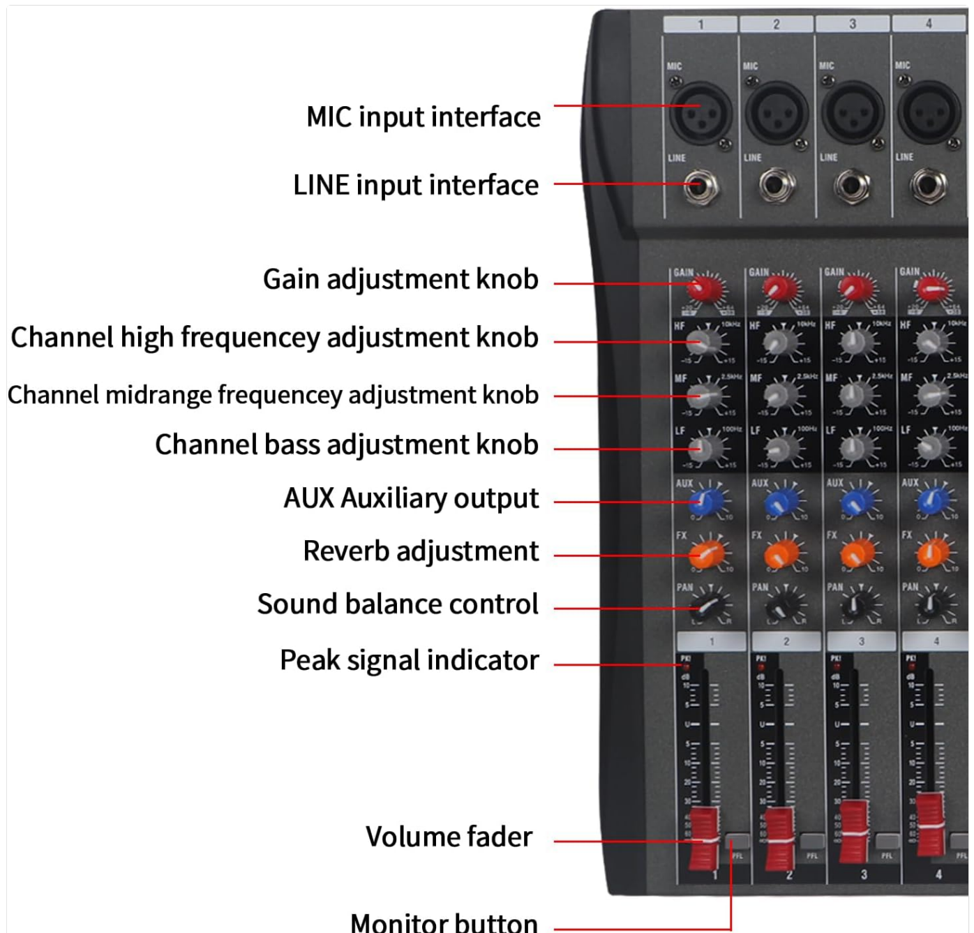
Image 4.1: Close-up of the input channels, showing MIC/LINE inputs, Gain, EQ, AUX, FX, PAN, PFL, and Volume Fader.
