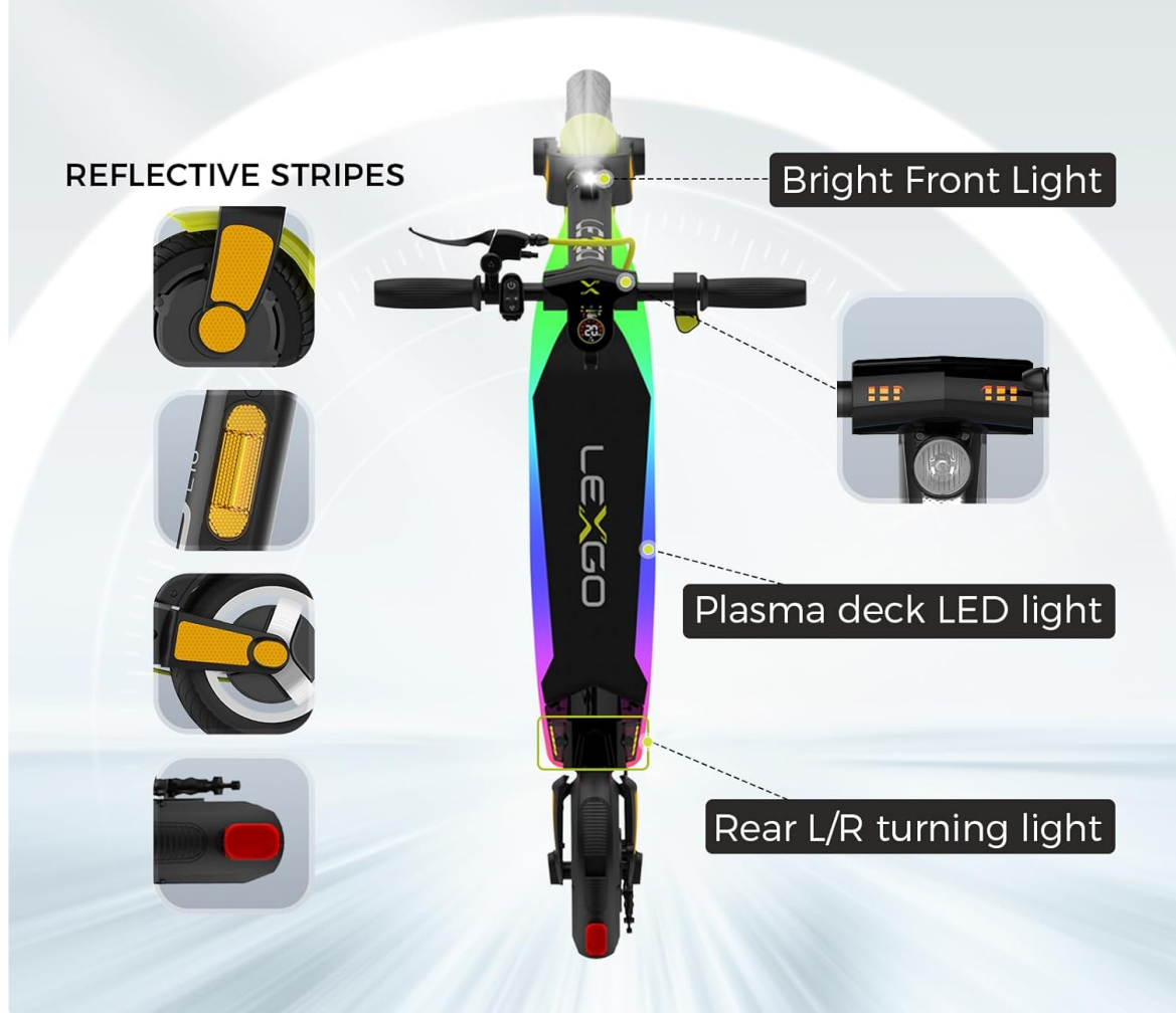
Figure 7: Safe Night Rides - highlighting reflective stripes, bright front light, plasma deck LED light, and rear L/R turning light.
