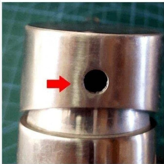
Image 2.1: Visual guide for installing the hot/cold indicator into a faucet handle.
