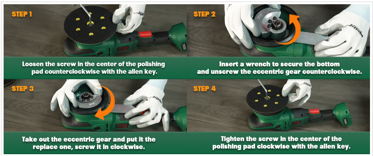
Image 4.2: Step-by-step guide for changing the polishing pad.
