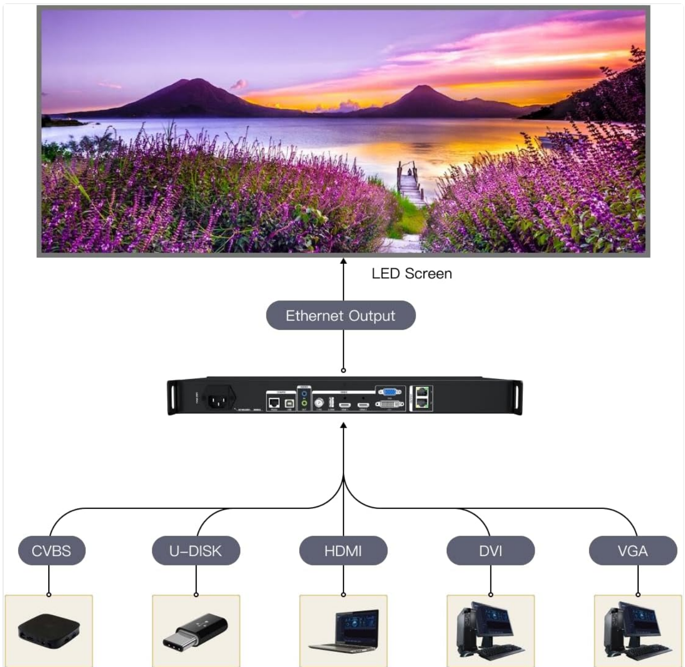
Figure 4: Diagram illustrating the typical connection flow from various video sources (CVBS, U-DISK, HDMI, DVI, VGA) through the X2m controller to an LED screen via Ethernet output.
