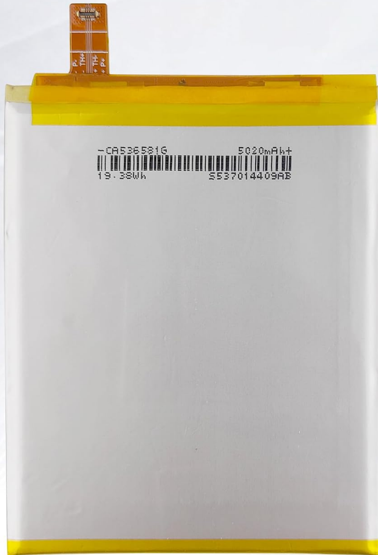
Image: The reverse side of the LK50 battery, displaying its model number, capacity, voltage, and various regulatory compliance markings.
