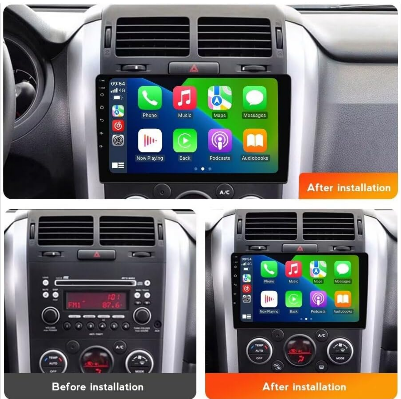
Figure 4.2: Visual representation of the car's center console before and after the installation of the Biorunn Android 13 Car Stereo, demonstrating the integrated fit.
