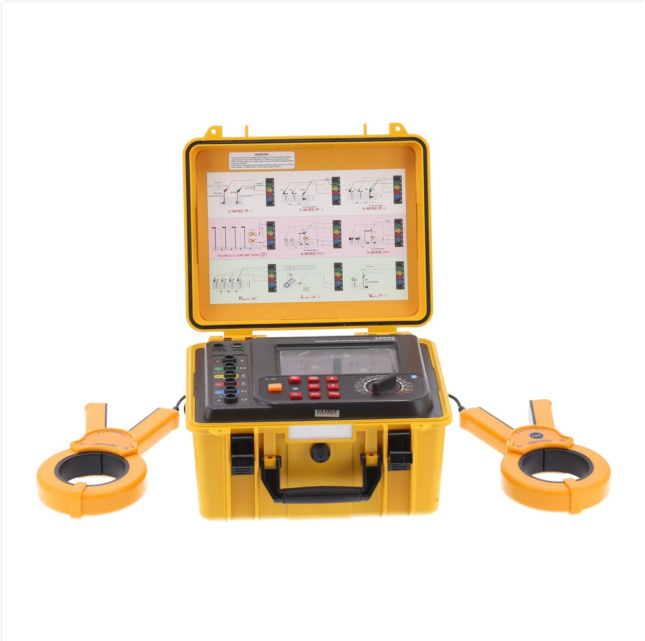
Image 5.2: ETCR3200C with current clamps for AC current and double clamp testing.
