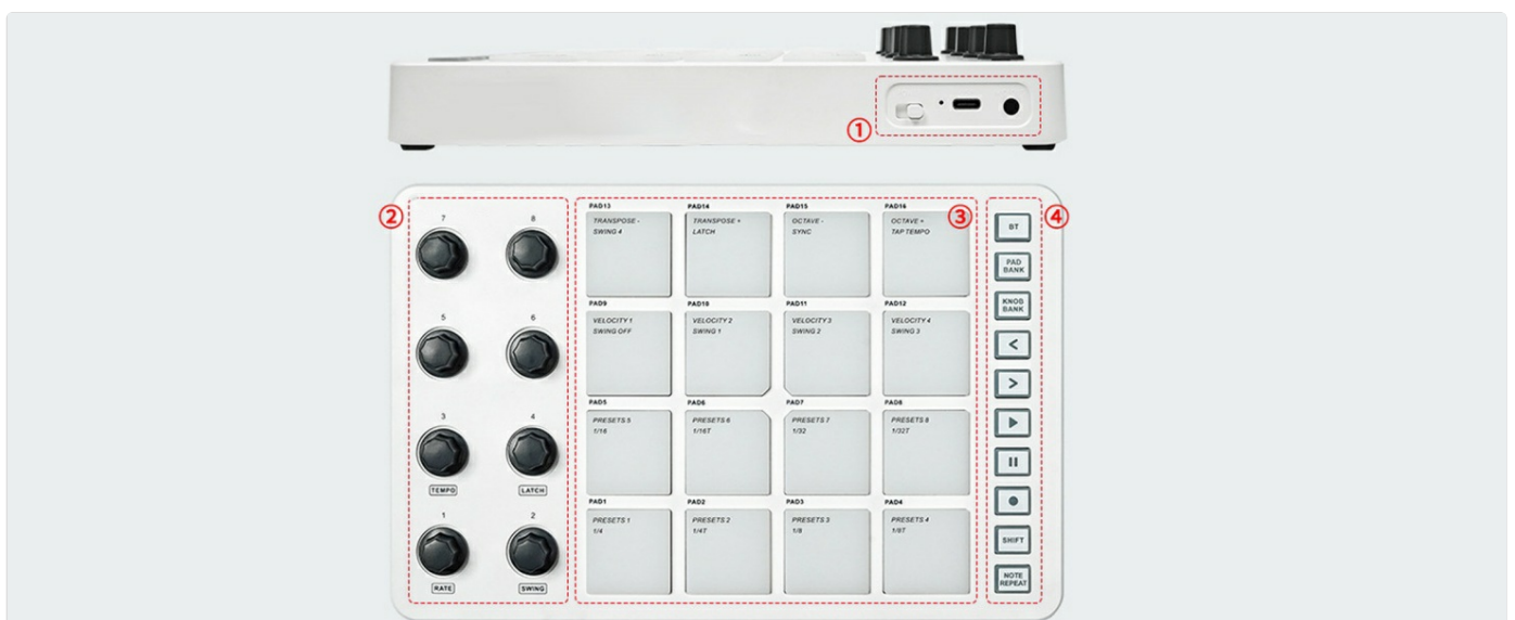
Figure 4.2: Labeled diagram of the MIDI Pad Controller's main components.
