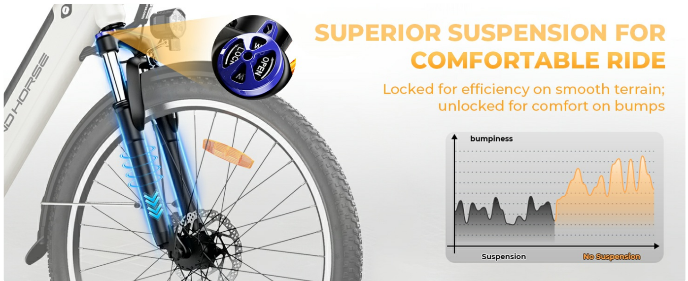
Image: The front suspension system, illustrating its ability to absorb impacts for a smoother ride.
