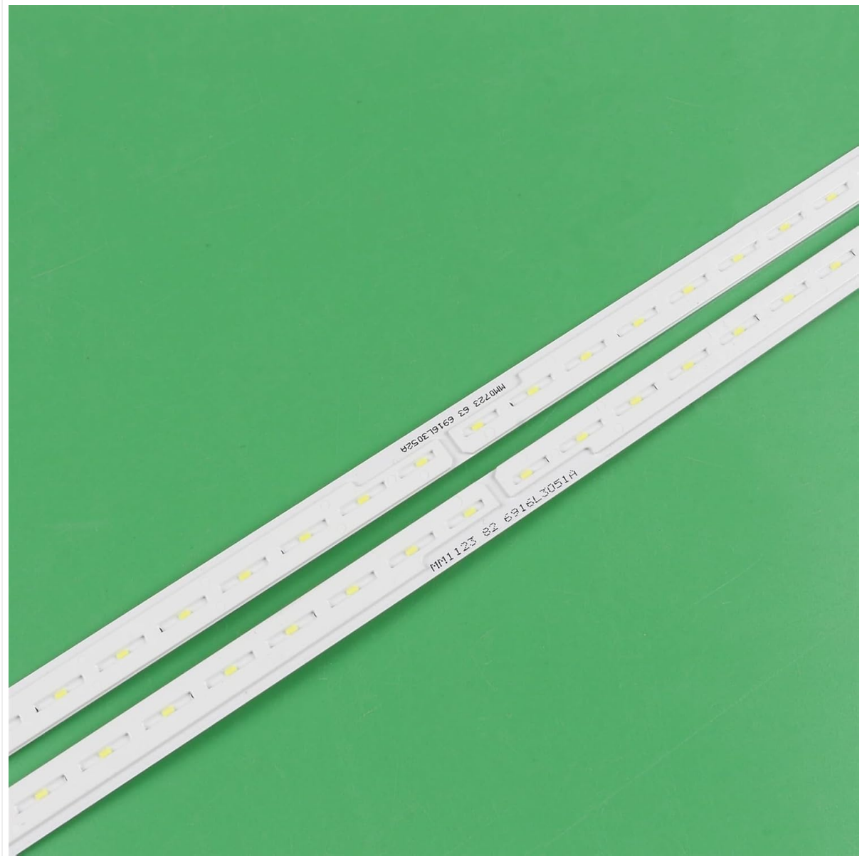
Image 4.1: Detail of the LED strip, highlighting the part number for verification.
