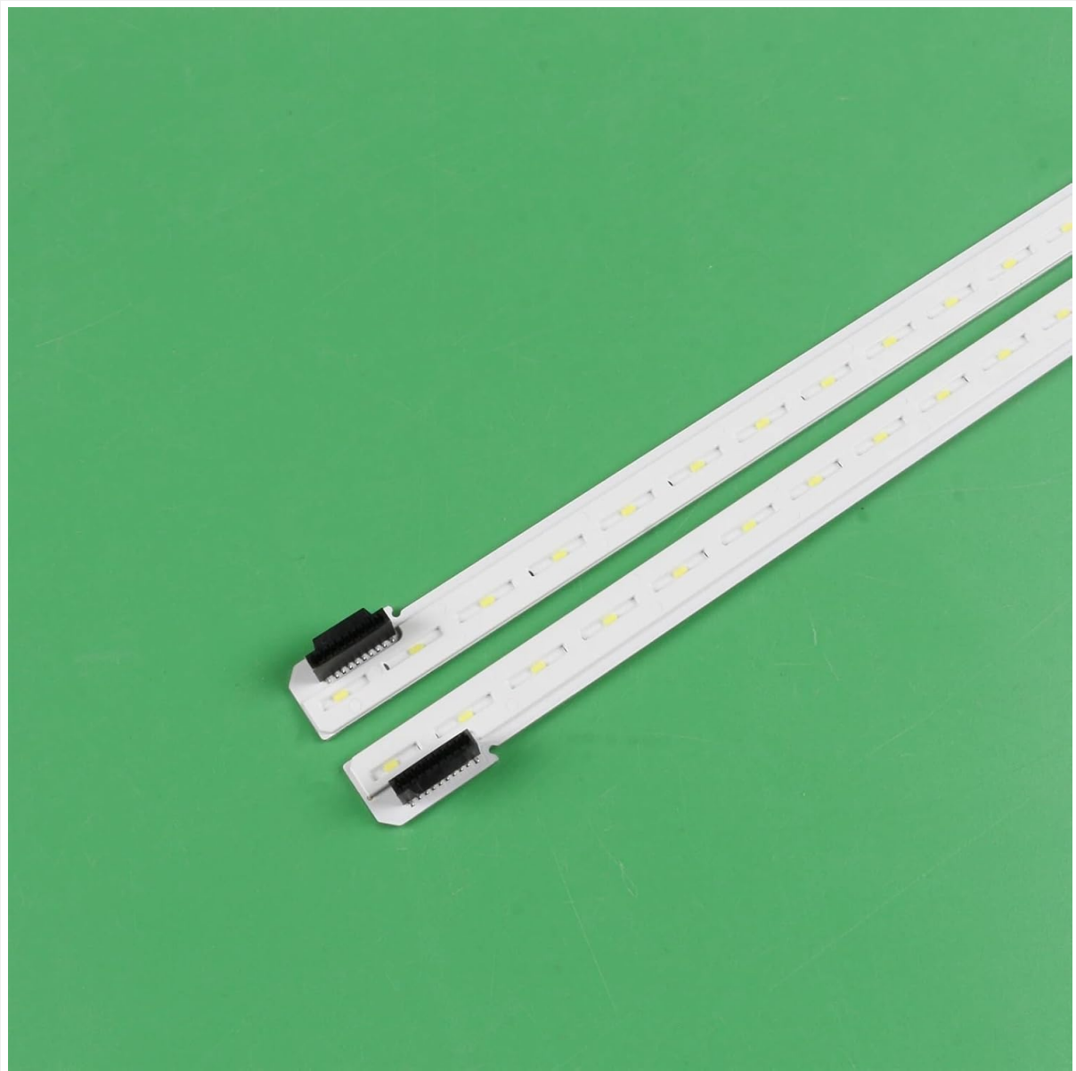
Image 5.1: Detail of the strip's connector, which should match your TV's existing wiring.
