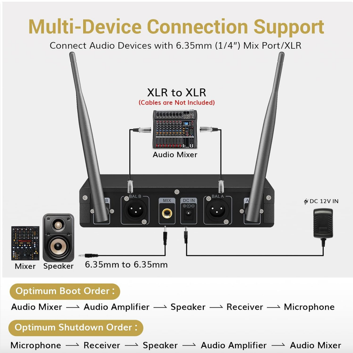
Figure 4.1: Connection diagram illustrating how to connect the receiver to an audio mixer, amplifier, and speakers using 6.35mm or XLR cables. Note that XLR to XLR cables are not included.
