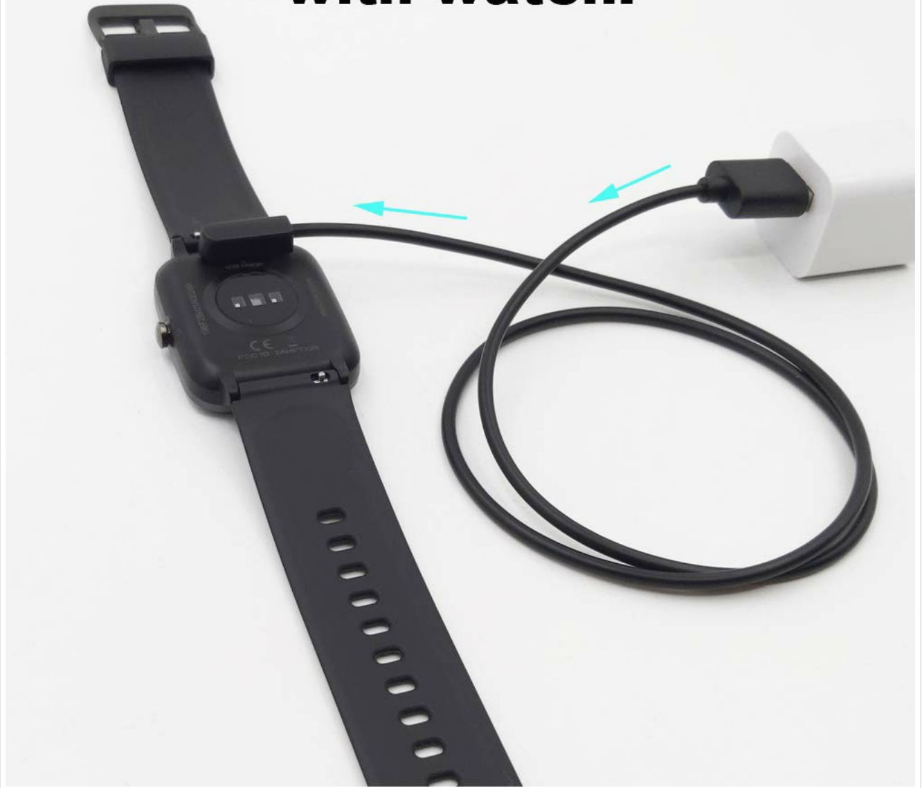
Figure 4.1: Charging the smartwatch using the magnetic suction connection.
