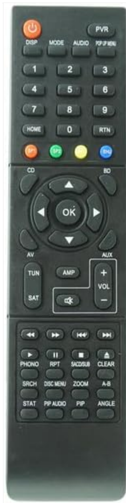
Image 2.1: Front view of the Generic replacement remote control. This image displays the full button layout, including power, numerical keys, navigation, volume, and various function buttons for audio and video control.
